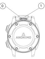
Position 0: The watch is working and water resistance is guaranteed. The crown is locked thanks to the patented protective lever.
